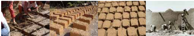
Process made from sand, clay, and water, with some kind of fibrous or organic material (sticks, straw, dung), which is shaped into bricks using frames and dried in the sun.
